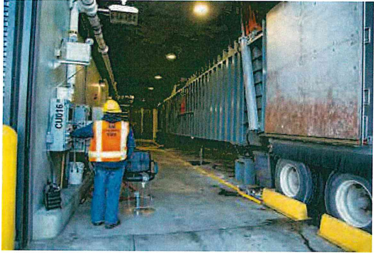
Compactors at the Factoria Recycling and Transfer Station compact trash, reducing the number of trips that county transfer trucks make to Cedar Hills
