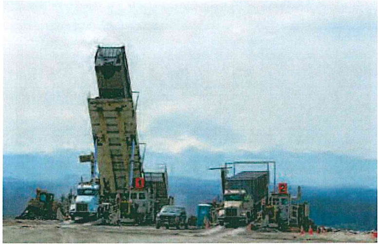
Tippers empty trailers more efficiently
